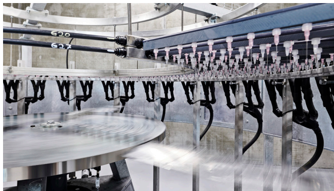
620 nozzles simulate realistic rainfall with adjustable droplet size.
