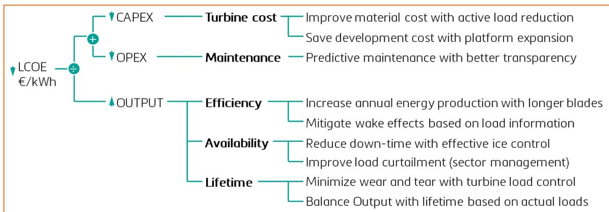
Figure 1 shows examples of the various levers that can be pulled to bring down cost of energy by utilizing rotor blade sensors. Driver tree to reduce levelized cost of energy (LCOE) with applications that make use of rotor blade sensing. CAPEX reductions immediately affect our customers' bills-of-material and R&D cost. Applications that reduce OPEX and those that increase output enable digital business models over the turbine lifetime.
