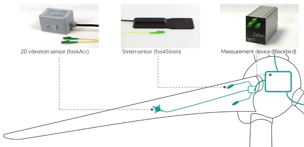
Figure 1: The modular fos4Blade IIoT sensor set consists of a central measurement device with 1-5 measurement channels per blade and an application specific combination of fiber-optic strain and vibration sensors in the blades.
