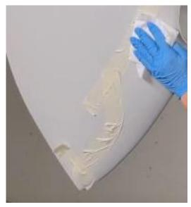
Apply a thin layer of adheson promoter  $3M^{m}$  **W9910-1** on the blade using a damp lint-free cloth.
