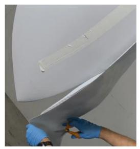
Dry fit the  $ELLE^{TM}$  Onshore to the TIP and evaluate how close to the TIP you can get. The  $ELLE^{TM}$  Onshore must be installed as far out towards the TIP – end as possible without creating waves on the sides that are **too** large to be smoothed out **during** installation. The TIP template can be used to trim the  $ELLE^{TM}$  Onshore if you want to install **further** out towards the TIP end than the waves on the sides allow.
