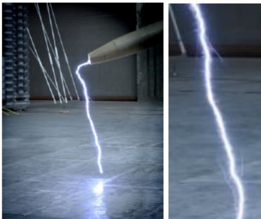
Figure 9: Picture from Initial Leader Attachment Test performed on a blade.
