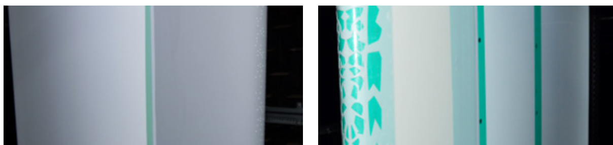
Figure 9 The 300 \mu\text{m} (top left) and 600 \mu\text{m} (top right) indentation were used within the wind tunnel test.
