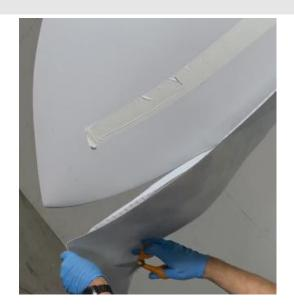
Dry fit the *ELLE®* Onshore to the TIP and evaluate how close to the TIP you can get. The *ELLE®* Onshore must be installed as far out towards the TIP – end as possible without creating waves on the sides that are too large to be smoothed out during installation. The TIP template can be used to trim the *ELLE®* Onshore if you want to install further out towards the TIP end than the waves on the sides allow, but you can also make your own tip cut design.
